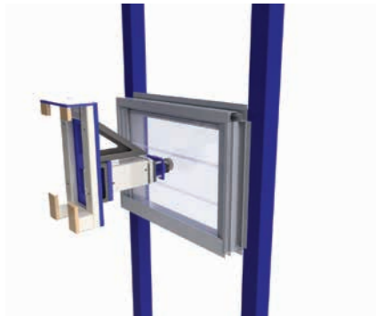
Load test in closed position
